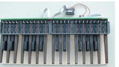
The two bass pedals can be mounted on a common base, e.g. made of wood. On the left side the bass pedal with the removed upper key is mounted. In the rear area the pedals have to mounted about 8-10 mm higher to have sufficient lift for the vertical movement of the keys. For this a small board (about 12 cm width and 10 mm thickness) over the whole lenght can be used (about 93,5 x 12 cm for two pedals).
