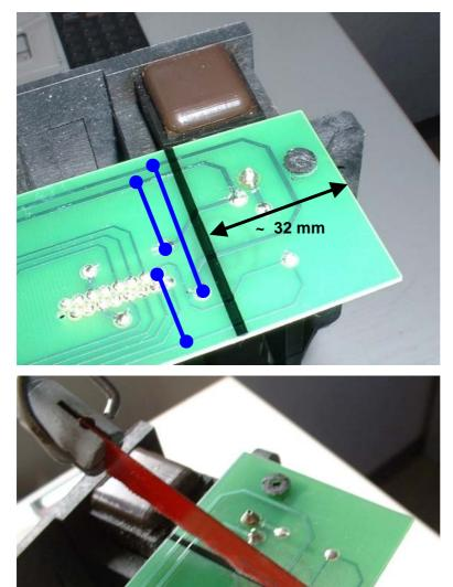
Mark a cutting line with a distance of about 32-34 mm from the pcb edge to the bottom of the pcb.
