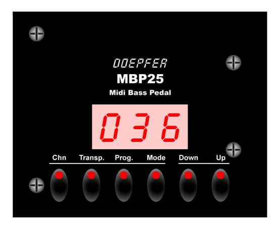
The three-digit display is used to show the value of the currently selected parameter, i.e. midi channel, transpose, program change number or mode. The LEDs indicate the currently selected menu.
