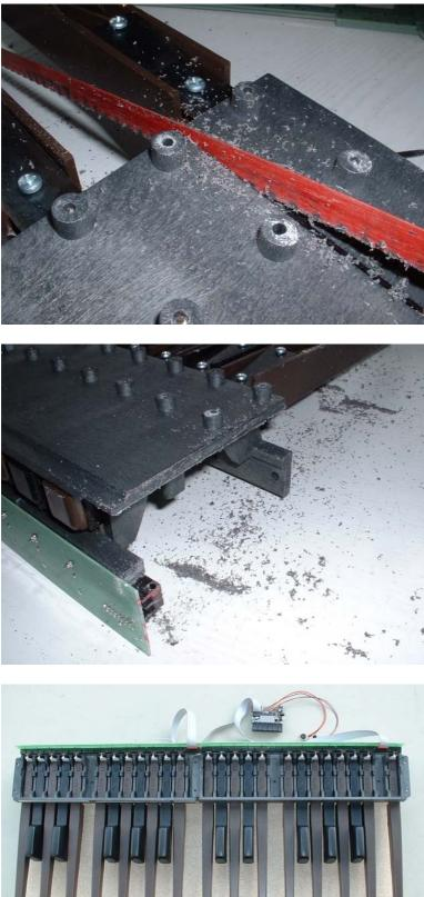
Cut off the pedal frame at this line with a suitable saw.
