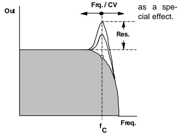
Fig. 1: Frequency response of the A-103
