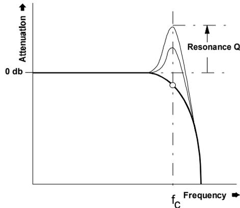
**Fig. 2:** How resonance affects the response of a filter around the cut-off frequency.
