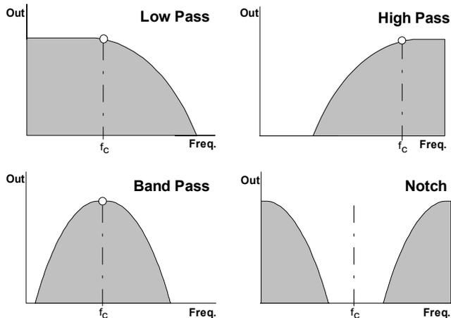
**Fig. 1:** Typical response curves of the four filters.
