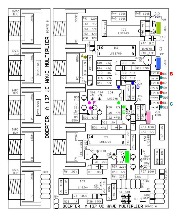
Correlation of measuring points and trimming potentiometers
