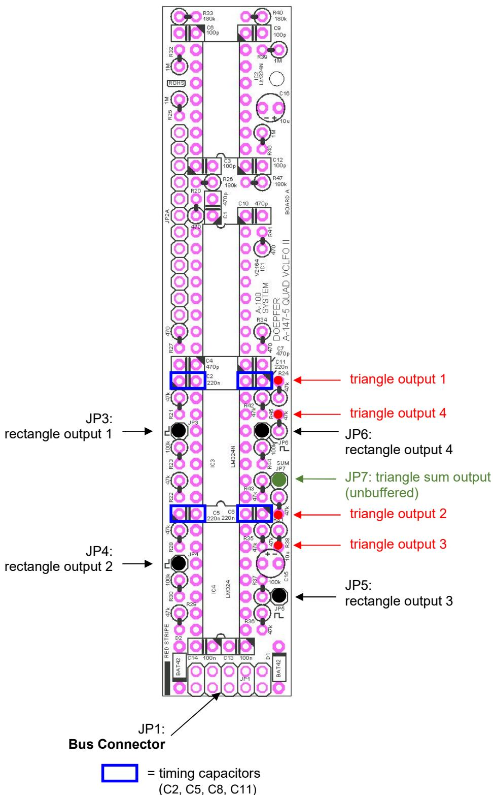
The timing capacitors can be replaced to obtain other frequency ranges. The factory value is 220nF.
