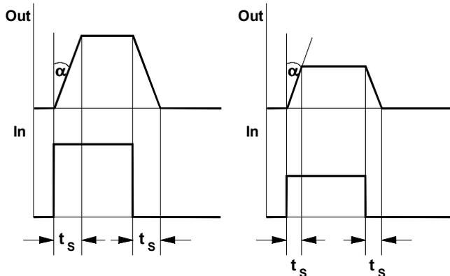
**Fig. 1:** How the A-171 transforms a signal.
