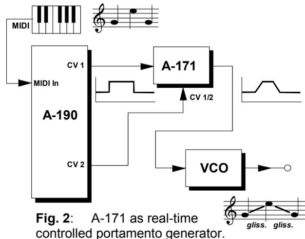
**Fig. 2:** A-171 as real-time controlled portamento generator.
