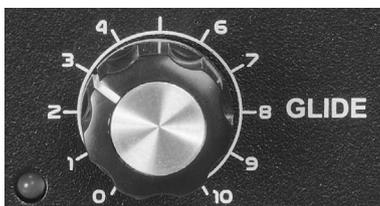
A popular effect is letting one note's pitch slide gradually to the pitch of the note played next. This function is also part of Dark Link. Synthesizers that do not feature this function can now easily be tricked into doing it without any further modifications necessary.
